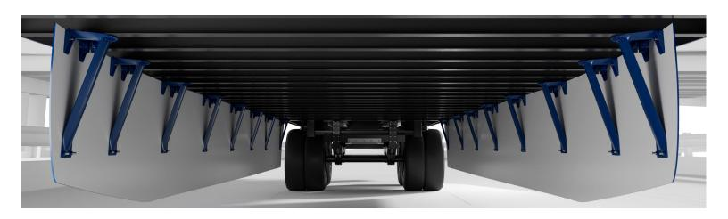
A revolutionary bracket system for EDGE SKIRTS® that is made to bend but never break.
