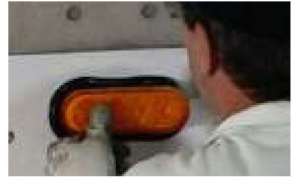
c. Install the light and connect all wires
