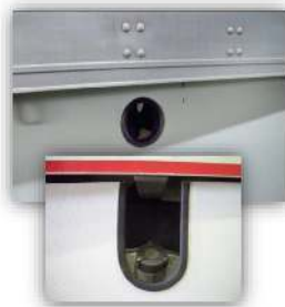
b. Place the trim seal provided by Transtex around the opening in order to protect its edges.
