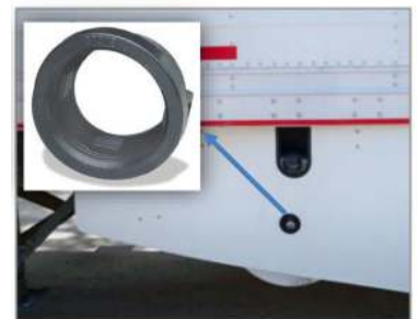
c. Use a 2 3/4" hole saw to make a round opening for the gage indicator. Insert the 2.5" round seal provided by Transtex.
