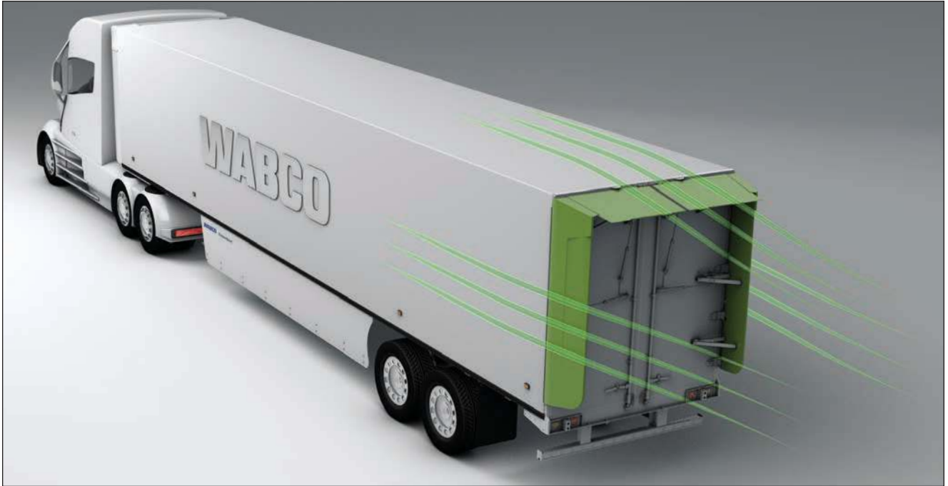
Similar to side skirts, rear trailer fairings improve trailer aerodynamics and allow customers to generate a return on investment in less than two years.
