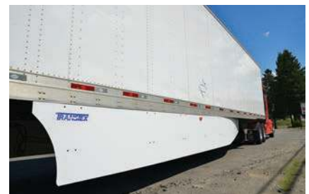
Aerodynamic trailer skirts provide major fuel economy benefits and can be installed in just a few hours.
