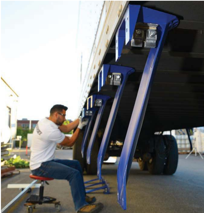
Aerodynamic trailer skirts provide major fuel economy benefits and can be installed in just a few hours.
